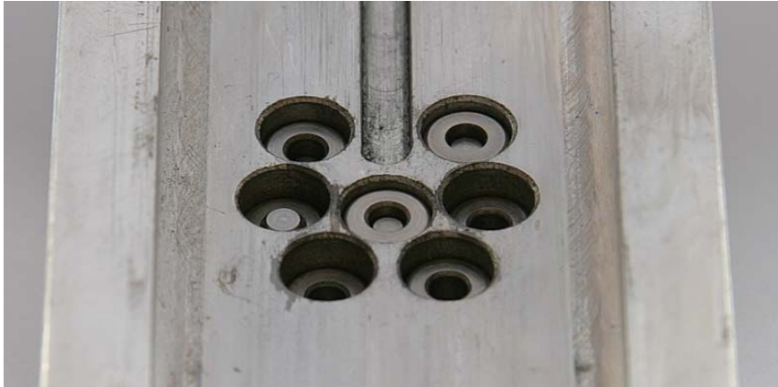
Shear line in back of Sliding front in locked position
